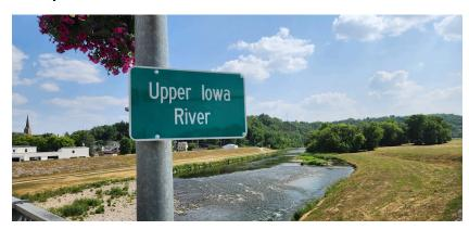
**Sign Locations:** Creek and river signs (and dual signs) should be installed in both directions of the road (a sign pair) at a creek or river bridge, preferably on the right side of the road in front of the bridge guardrail, as approved by the county engineer (on county roads) or by the city public works department (on city roads). Watershed signs should be installed at the river watershed divide at the entrance to the watershed (one direction of the road).
